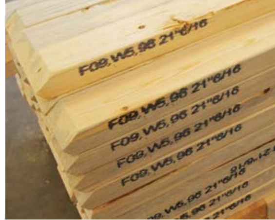
EVERY PIECE OF WOOD COMING OUT OF NVF IS CODED USING AN INKJET PRINTER SO THAT BUILDERS KNOW EXACTLY WHERE EACH PRECISION-CUT PIECE OR SECTION GOES.
