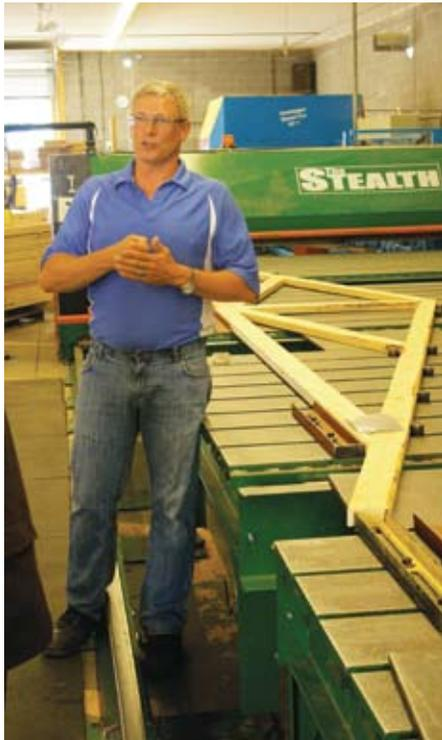
**MARK IBBETSON, OWNER OF NORTH VALLEY FRAMEWORKS, STANDS NEXT TO THE AUTOMATED SAWS THAT MEASURE AND EXTRACT EVERY PIECE OF USEABLE WOOD DOWN TO FIVE-AND-A-HALF-INCH SCRAPS.**
